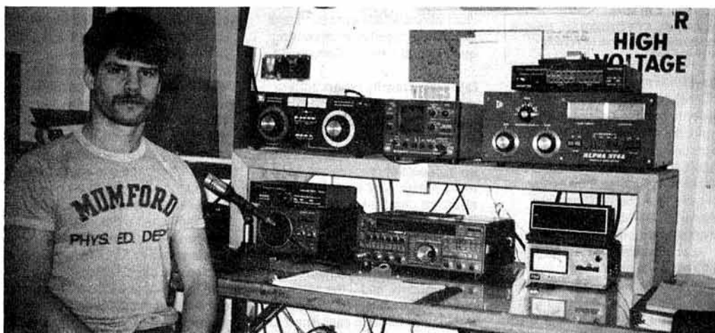
The shack at VE8RCS showing Mike Parent at the operating position. The station comprises an FT767GX, a Nye Viking ATU, a Kenwood 220 Station Monitor, plus phone patch equipment.
